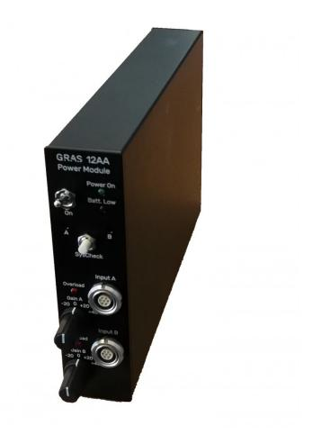
Connection:Traditional 200 V Channel(s): 2 The GRAS 12AA Power Module is a dual channel power supply for preamplifiers used with condenser microphones. It is for general use in acoustic measurements as well as for intensity measurements; both in the laboratory and in the field.
