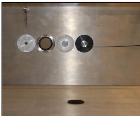
Figure 7. An overview of the setup in the small wind tunnel. From left to right are the following: 47BX (1/4" flush-mount); 67TS (Turbulence Screen); 47AX (1/2" flush-mount); and 40LS (surface microphone). The flow was equally from left to right. In the top is seen a 40SC probe microphone (whose results have not been presented herein); in the bottom is the opening of the sound source, mouth simulator 44AA.
