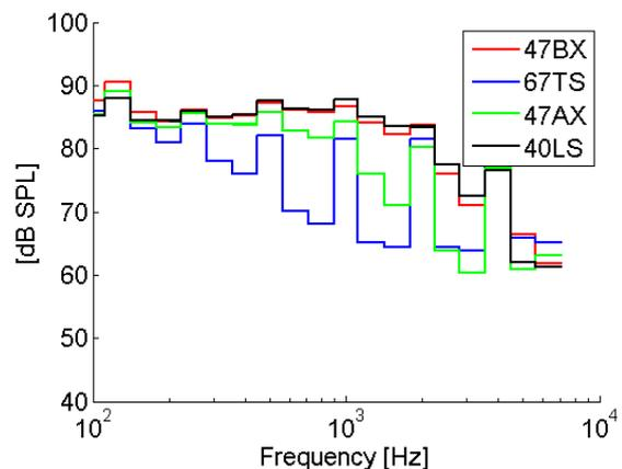
Figure 9. Response of the 4 transducers to the same multitone of pure tones as shown in Figure 8, though with added turbulent noise due to a free-stream velocity of 20m/s. The 67TS flush-mount Turbulence Screen clearly extracts the excited pure tones.
