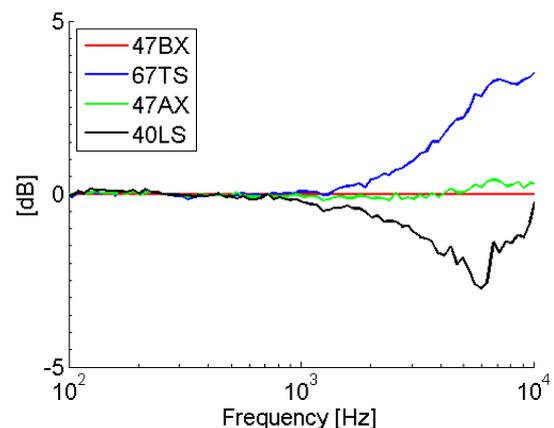
Figure 5. Pressure response of the transducers, relative to that of the 47BX, placed in a baffle and with sound arriving head-on.
