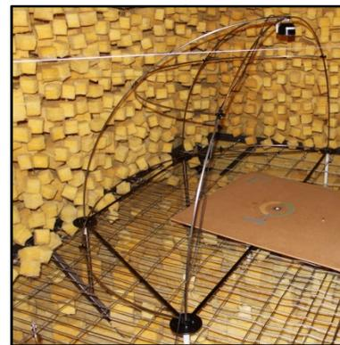
Figure 4. An overview of the setup in the anechoic chamber. The sound source, seen in the top, was placed on a  $\varnothing 2$ m hemisphere. The transducers were flush-mounted in the baffle shown below, centered at the origin of the hemisphere.
