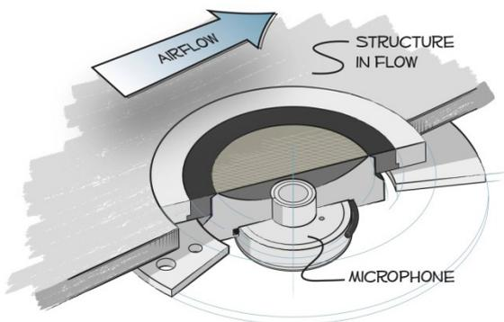
Figure 3. Schematic of flush-mount Turbulence Screen, 67TS.
