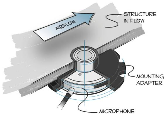
Figure 2. Schematic of flush-mount microphone, 47BX.
