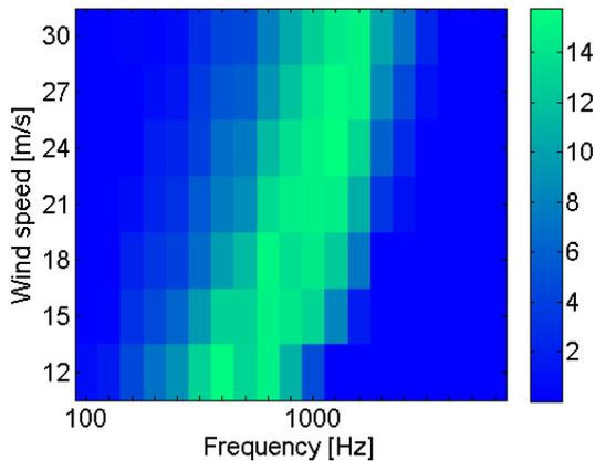
Figure 10. The attenuation of a 67TS flush-mount Turbulence Screen relative to a 1/2" flush-mount 47AX (in dB), measured at various wind speeds in a small wind tunnel. The effective frequency range of the 67TS changes with wind speed as the apparent size of turbulent eddies is reduced.
