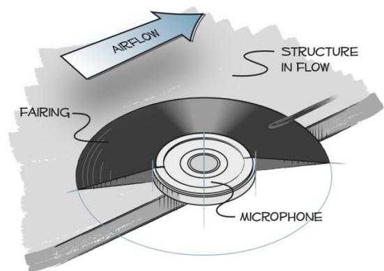
Figure 1. Schematic of surface microphone, 40LS.
