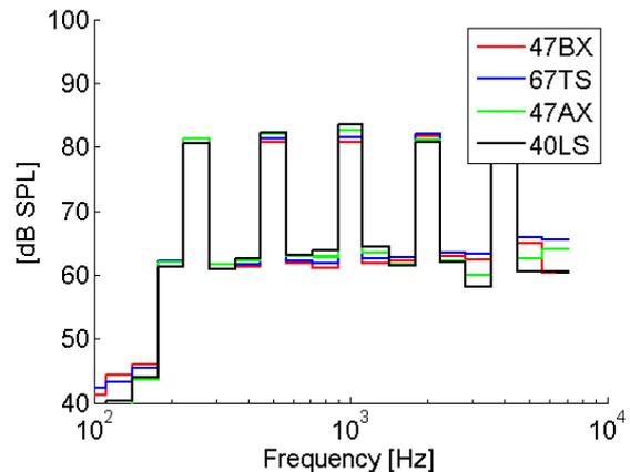
Figure 8. Response of the 4 transducers to a multitone of sinewaves (no air flow), displayed in 1/3rd octave bands. The deviations from one another is primarily caused by the differing placements (see Figure 7).
