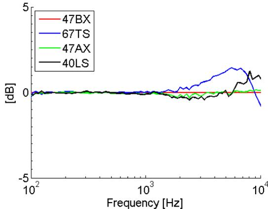
Figure 6. Pressure response of the transducers, relative to that of the 47BX, placed in a baffle and with sound arriving parallel to the plane of the baffle.
