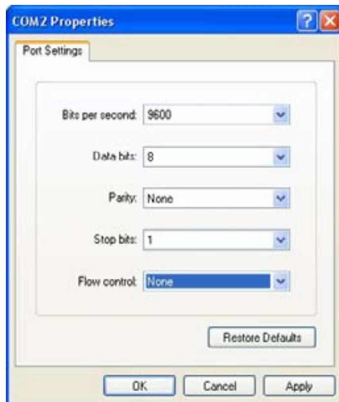
Fig. 4.3 Showing the correct setup for the selected COM port
