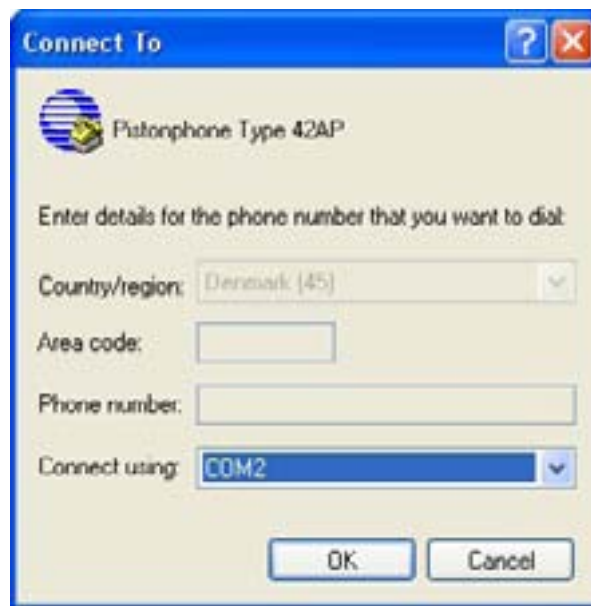
Fig. 4.2 Selecting the COM port in use, e.g. COM2
