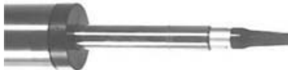
Fig. 3.3 ½" microphone inserted in the coupler
