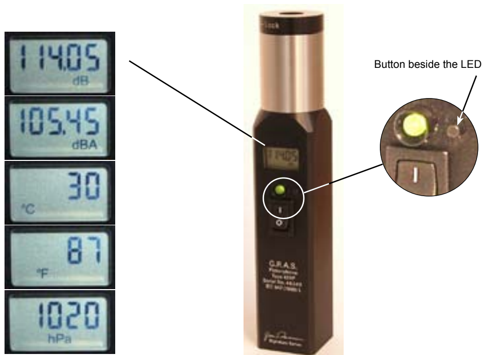
Fig. 1.1 Pistonphone Type 42AP shown with display examples
