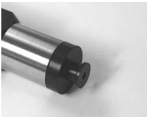
Fig. 3.5 \frac{1}{8} " microphone adapter inserted in the coupler
