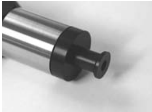
Fig. 3.4 ¼" microphone adapter inserted in the coupler
