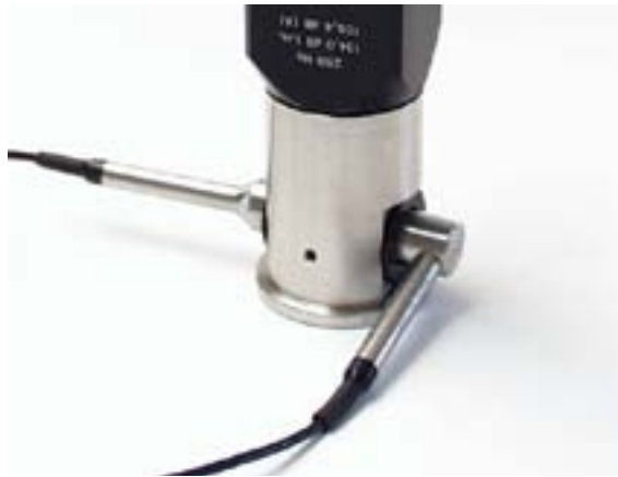
Fig. 5.1 Two-port Coupler RA0024 shown here with the two phase-matched microphones of an intensity probe
