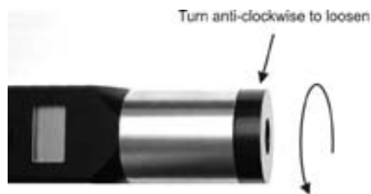
Fig. 3.2 Loosening the microphone retention collar
