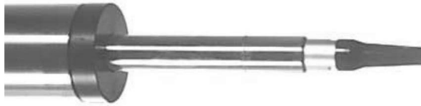
Fig. 3.3 1/2-inch microphone inserted in the coupler
