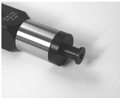
Fig. 3.4 1/4-inch microphone adapter inserted in the coupler
