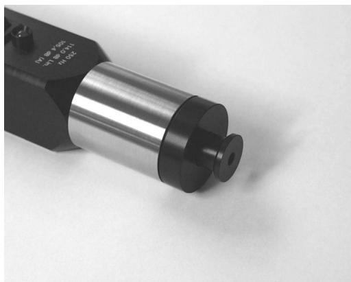
Fig. 3.5 1/8-inch microphone adapter inserted in the coupler
