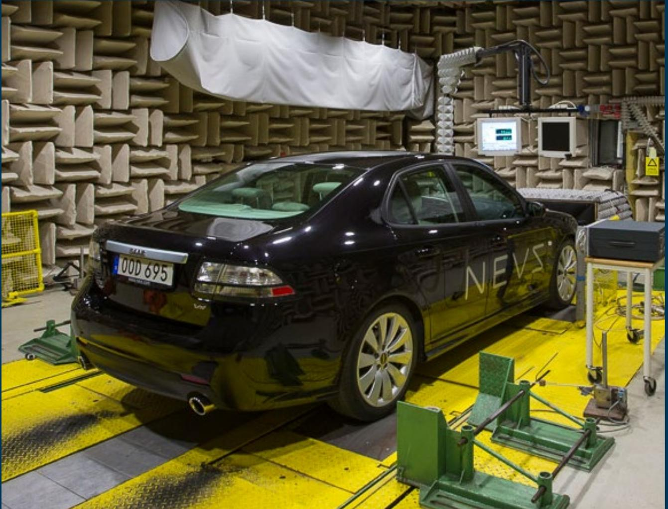
The exhaust noise from vehicles with internal combustion engines is very important. It must support a good engine sound quality while not being disturbing or violating noise legislation. The intake system and exhaust system are highly responsible for the engine noise character and sound pressure level (SPL) and must be tuned to meet the required performance. The engine
