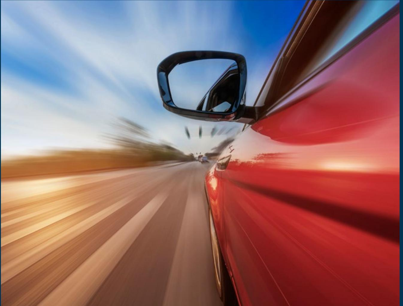
Wind noise is an aerodynamic noise related to the body design and turbulence from components such as side view mirrors, wipers, cavities, etc. It is most disturbing at speeds above 100 km/h (approx. 60 miles/h), but is becoming more and more important when powertrain and road noise is being reduced. Careful design minimizes the
