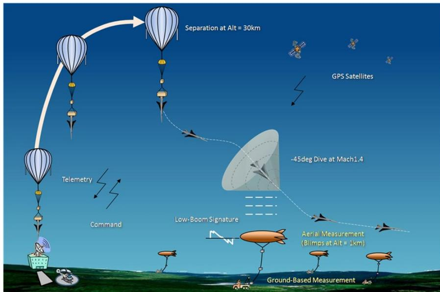
Figure 9. Test Setup for Drop Testing With Validated Instrumentation System
