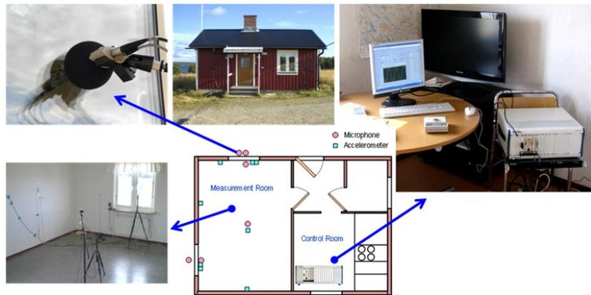
Figure 7. Test Setup for Sonic Boom Ground Test
