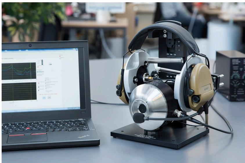
The GRAS 45CC-7 with ear simulator and ½" prepolarized measurement microphone and the T5 Invisio Headset.
