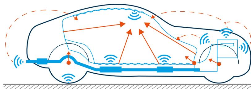
*The ATF is measured reciprocally with a noise source at ear position and the response in the engine bay.*
