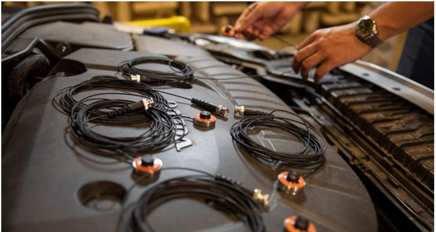
Since the 147AX operates in the -40 to 125 °C (-40 to 257 °F) temperature range and is designed to be water and dust proof (IP67), it will survive even the most challenging engine bay environments.
